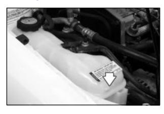
The surge tank is located on the passenger's side of the engine compartment.
